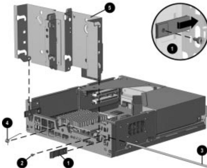
*Removing the Drive Cage*
