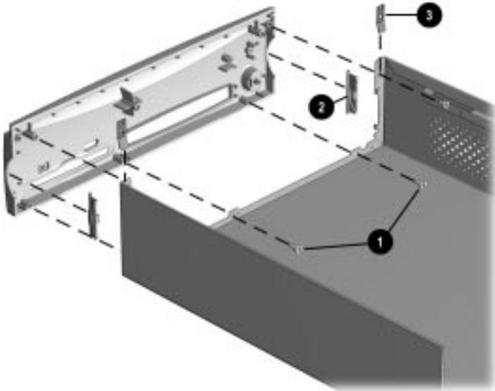
*Removing the Front Bezel and Cover Release Buttons (Small Form Factor shown))*
