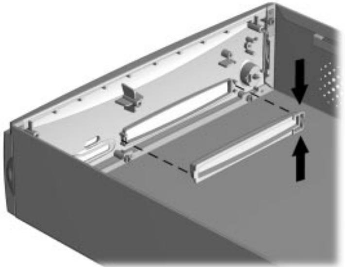
*Removing the Bezel Blank (Small Form Factor Shown)*
