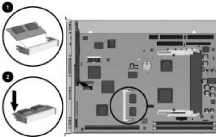
*Installing an Upgrade Memory Module*
