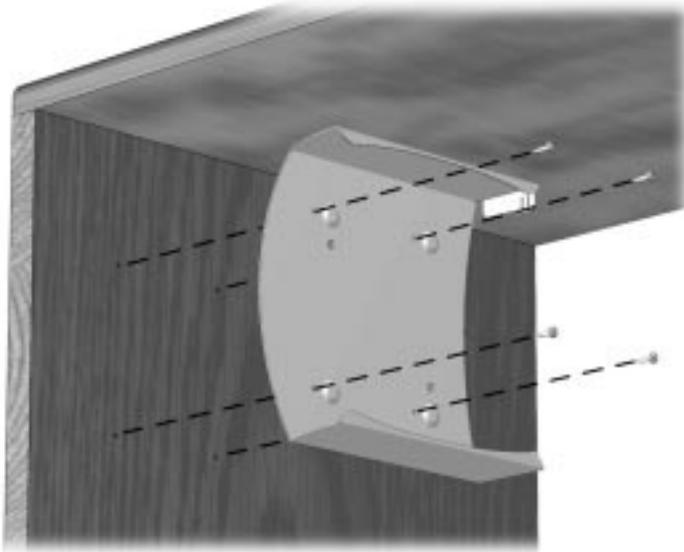
*Installing the Mounting Bracket in a Vertical Mode*
