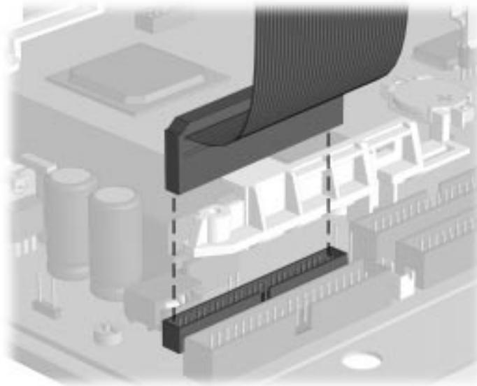
*Connecting the Flat Ribbon CD-ROM Cable to the System Board*
