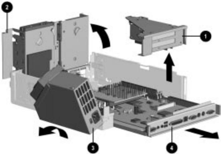
*Removing the System Board*
