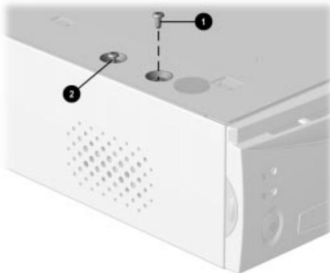
*Removing the Smart Cover Lock Screws*
