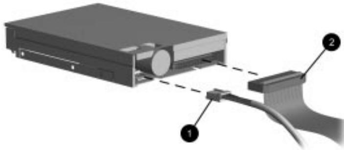
*Disconnecting the Power and Data Cables from the 3.5-Inch Diskette Drive*
