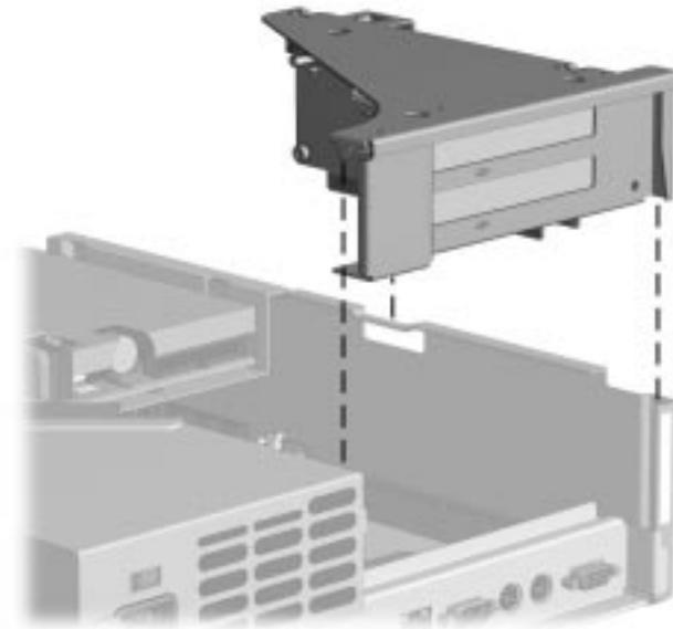
*Removing the Expansion Board Cage*
