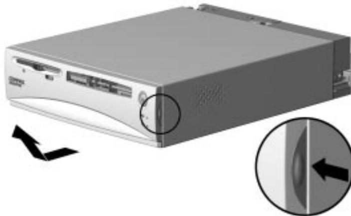
*Removing the System Unit Cover*
