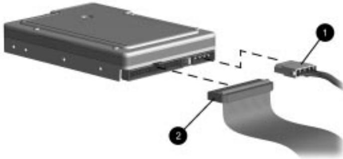
*Disconnecting the Cables from the Back of the Hard Drive*
