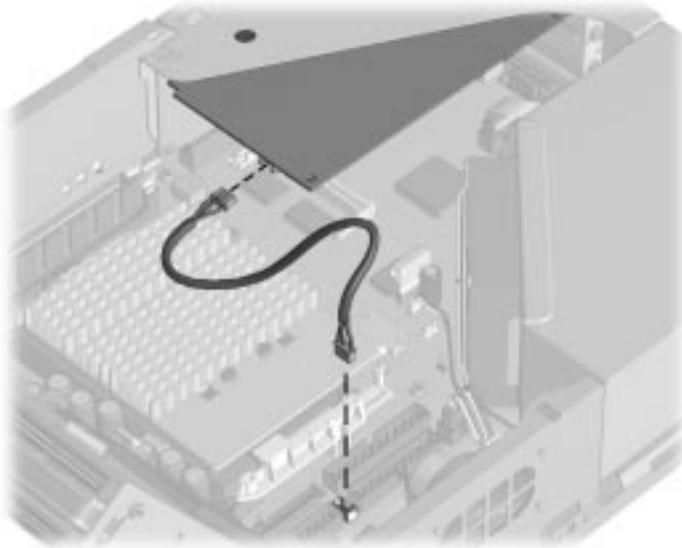
*Attaching the Audio Cable to the System and Audio Boards*
