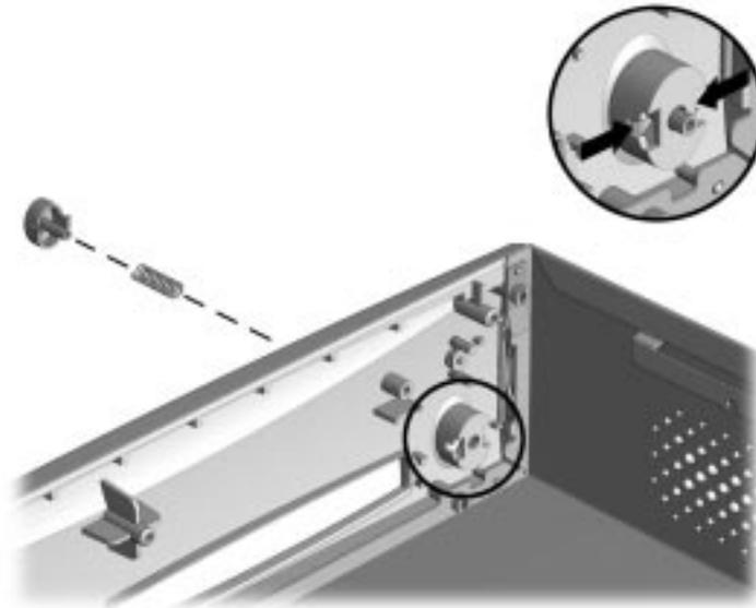
*Removing the Power Button (Small Form Factor Shown)*
