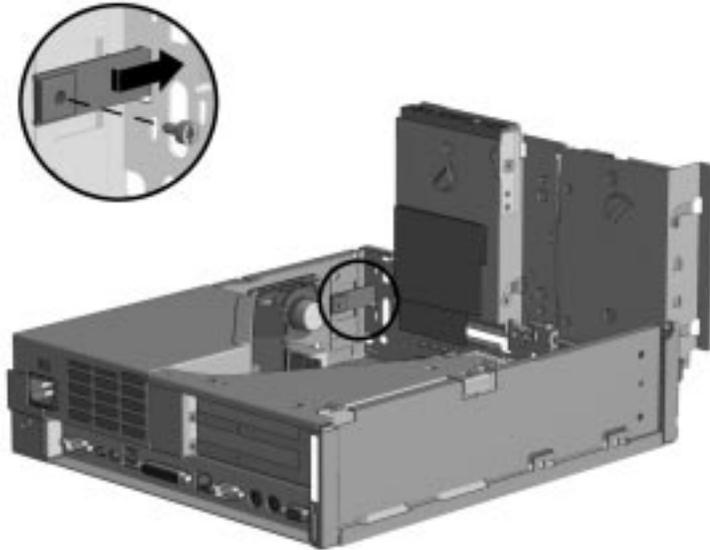
*Removing the Hood Latch Retainer*
