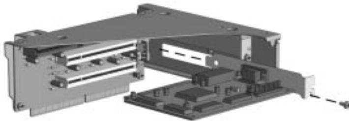
*Removing the Expansion Board*
